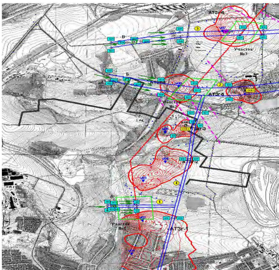
Fig.5. Contours of geoelectric anomalies of the ATZ and the boundaries of gas-permeable “channels” on topographic map of the mining allotment section of the A.F. Zasyadko coal mine [17].
