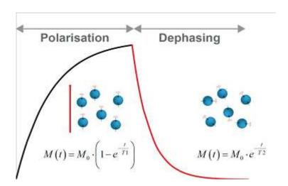
The peak magnetization detected when the hydrogen nuclei are fully polarized is a direct measure of how much hydrogen in present in the fluids in a rock, this in turn is a function of the water content or porosity. The rate at which the hydrogen nuclei polarize, characterized by the longitudinal relaxation time T1, and
