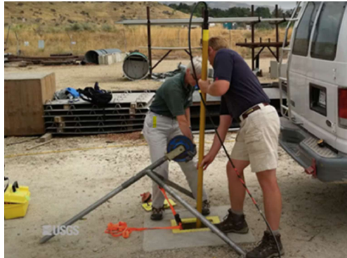
Figure 3: USGS scientists prepare to collect a nuclear magnetic resonance (NMR) log at a well (Source: USGS ).
