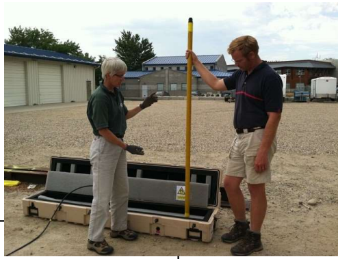
Figure 1. USGS hydrologists prepare a borehole NMR tool for logging ( Source: USGS ).
